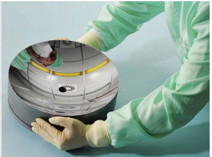
Fig. 3: Mo/Si coated EUV collector mirror for high-power LPP sources. R > 66.5 \% , \lambda = 13.500 \text{ nm} , Bandwidth of reflectivity at half maximum > 0.510 \text{ nm} , standard deviation of peak wavelength = 0.001 \text{ nm} (measurements: PTB Berlin, BESSY II).
